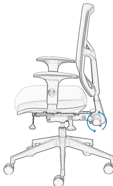
EN Adjusting the height of the backrest by locking the handwheel
