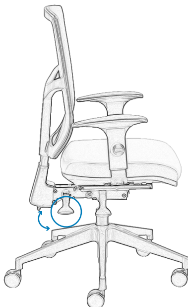
EN Adjusting the angle of the backrest by rear right lever
