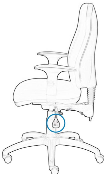
**EN** Adjustment of the tilt angle of the seat
