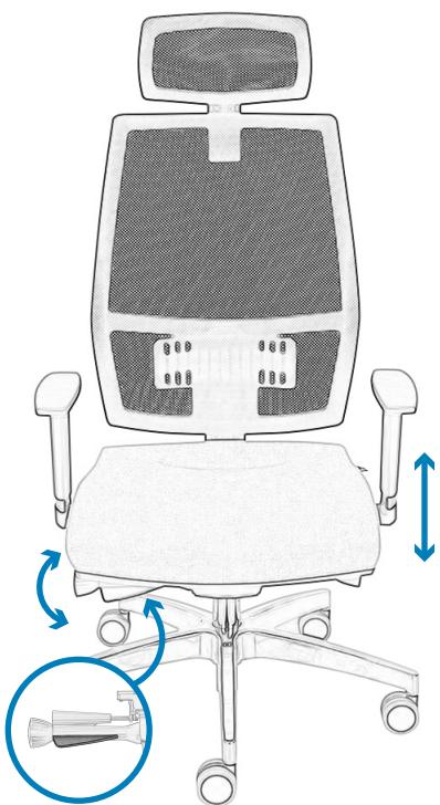
**EN** Seat height adjustment by means of the right lever
